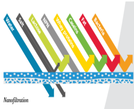
Fig 5: Nanofiltration of Milk
