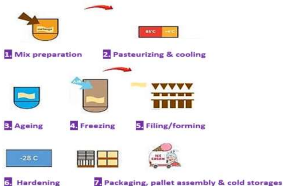
Fig 6: Ice cream Production flow chart
