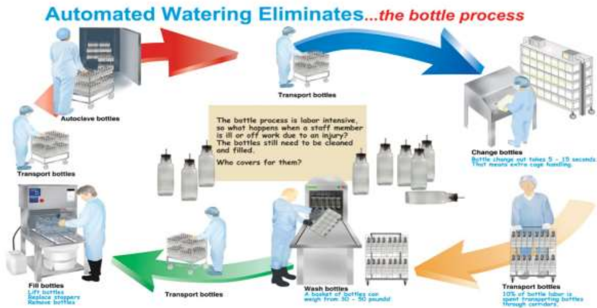
Fig 1: Bottle cleaning and filling Process
